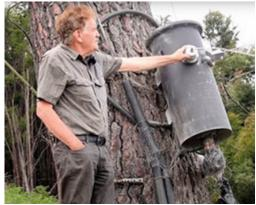
A huge 12:1 balun resembling a utility pole power step-down transformer converts the impedance from 50 W unbalanced to 600 W balanced. The wire he uses for each leg is aluminum-wrapped, power-line cable (10-millimeter cable with wrap), and he uses power-line fittings, because they're designed to handle the wire. The line has a 60-ton breaking strength.
