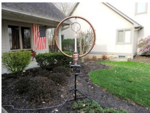
The magnetic loop for 40 and 20 meters designed by Richard Robbins, WA8RR. [Photo courtesy of DELARA News ]
