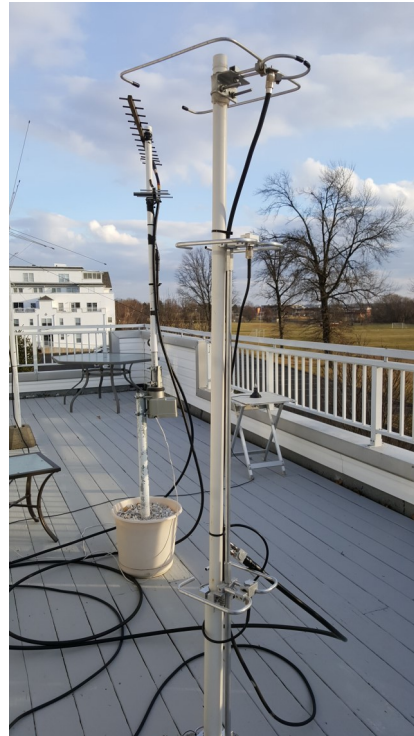
This shows a pvc pipe with the dual band 2/440 squalo halo. Underneath is the stacked 222 squalos.
