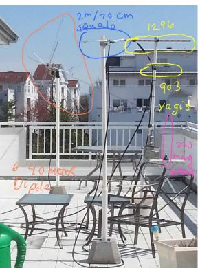
This is our aluminum farm. Each antenna is marked. We currently have 40 meters to 1.2 gigs. Hoping in the future to run 50+ feet of wire near the gutter hooked up to my smart tuner so I can get in on 80 mins. We accept any and all suggestions.
