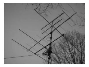
This is my collection of borrowed antennas, mostly from Bill Shaw, K3EGE. From bottom to top: a 3 element 6 meter beam, a 222 MHz loop; a 2 meter Yagi, a 432 MHz Yagi, and a portion of a 1296 MHz looper. Not shown is a copper pipe 222 MHz J-pole borrowed from KA3FQS that I raised up in a nearby tree using my Al Konschak-inspired slingshot. I was short on coax but K1DS, KA3FQS, and Dave Fle mming, KB3HCL, came through with some extra lengths.
